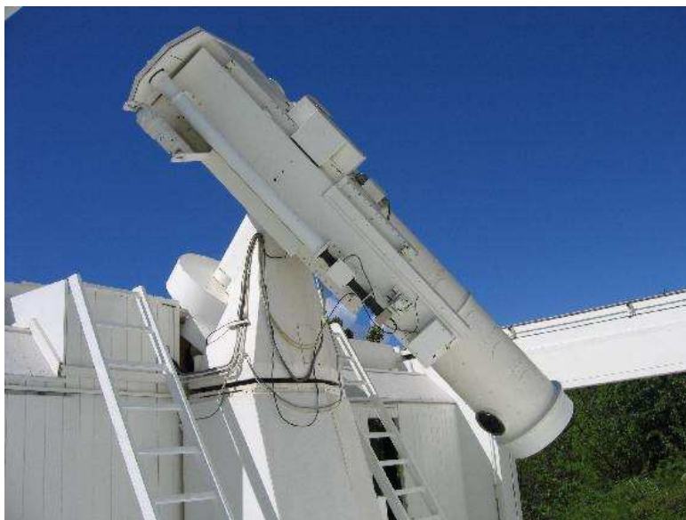
Fig. 2. The 45 cm aperture Gregory Coudé vacuum telescope.
