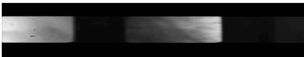
Figure 6. Sample image of H- \alpha showing an image with the wavelength 6563.3 Å in the middle and two adjacent ghost images at 6563.3 \pm 3.74 Å
